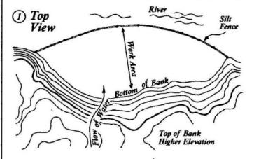
Prepare a stormwater pollution prevention plan. Set up silt fences according to terrain, soil and run-off consideration. Prevent soil migration by decreasing soil exposure, steep unvegetated slopes and construction time. Revegetate as soon as possible in the SAME SEASON.
